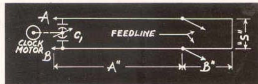
Fig. 4. Schematic diagram of the matching stub for use with untuned feedlines. The spacing "S" is about 1 inch. For 72-ohm twin lead, dimension "A" is about 18 inches, and "B" is about 6 inches. The over-all stub length is the same for other feedlines, but the tap position may change.
